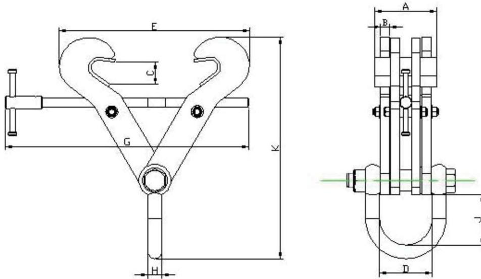
The Jumbo Beam Clamp is a great option for rigging applications. This clamp line features a wide jaw opening for wide flange beams used throughout industry. The JBC's clamp screw assembly is also zinc plated. This clamp series features metric capacities that range from 3, 5, 6, 10 and 16 tons.
