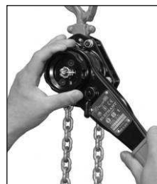
5) Hold down the feed handle softly and manipulate the operation handle to pull the bottom hook.
