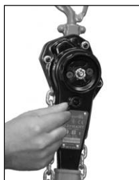
4) Set the selector lever to "UP" position.
